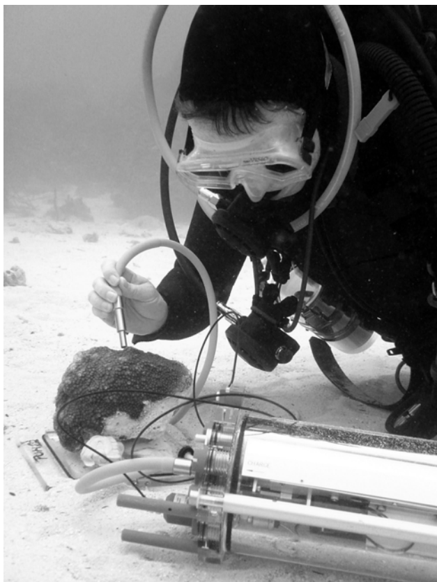
VIMS graduate student Jo Gascoigne uses a fluorometer to measure the photosynthetic ability of the algae that normally inhabit coral tissue.
