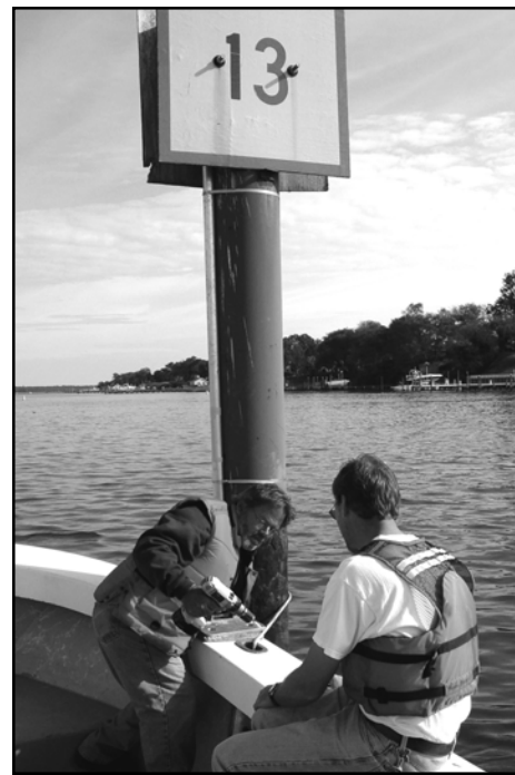
VIMS Laboratory Instrument Maker Wayne Reisner (L) and Lab specialist Tim Gass (R) attach a current-meter to a Lynnhaven channel marker.
