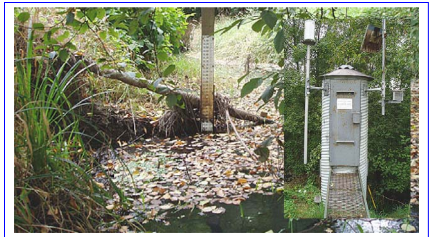
Figure 5.49 USGS monitoring station at Spring Brook Creek, WA. (Source: USGS Washington Water Science Center)
