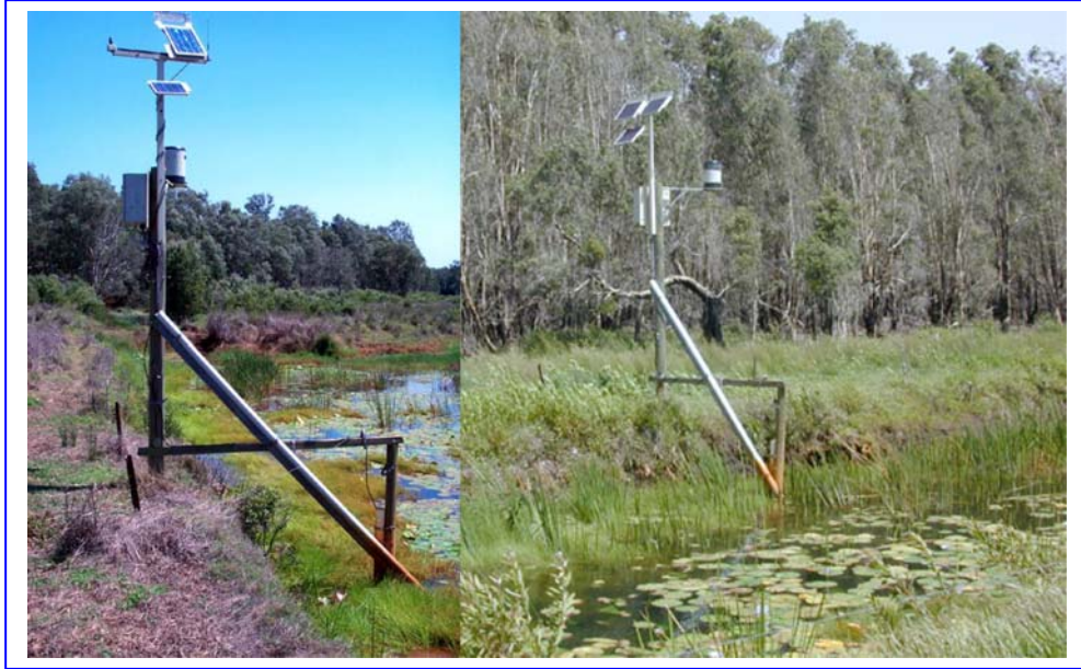
Figure 5.53 Wood post & steel pipe structure (Source: New South Wales Department of Natural Resources, Lower Richmond)
