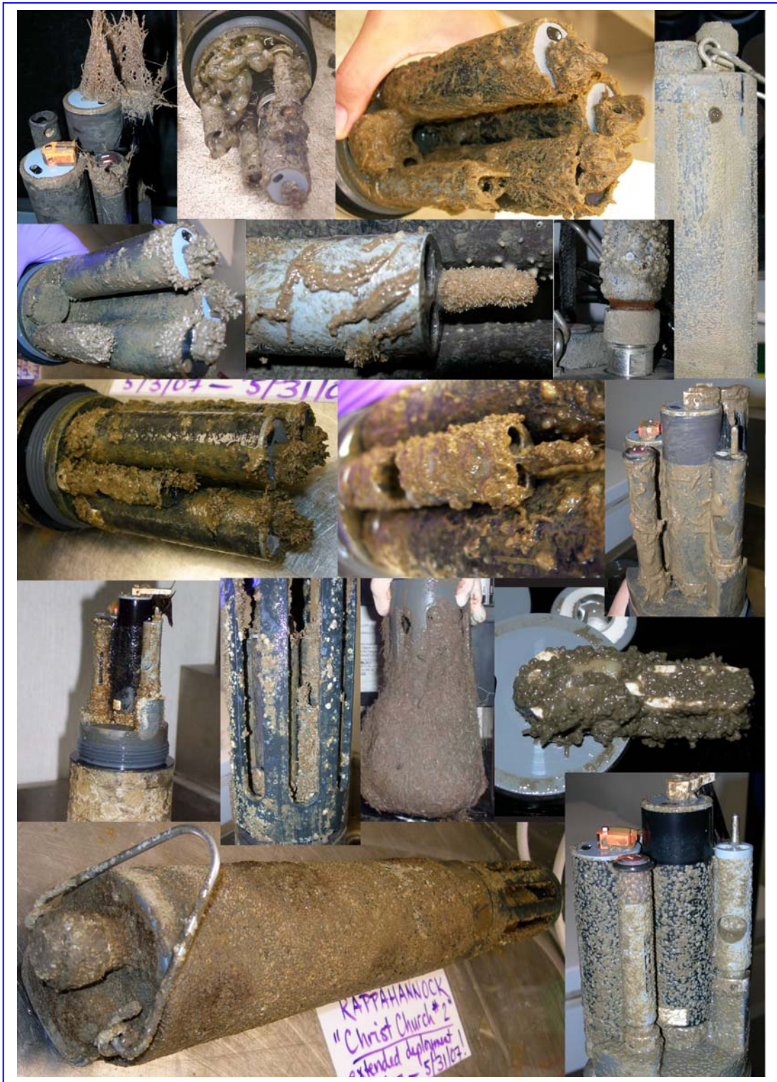
Figure 7.2 Biofouling examples (Source: CBNERRVA, NIW - NERR, CIORE)
