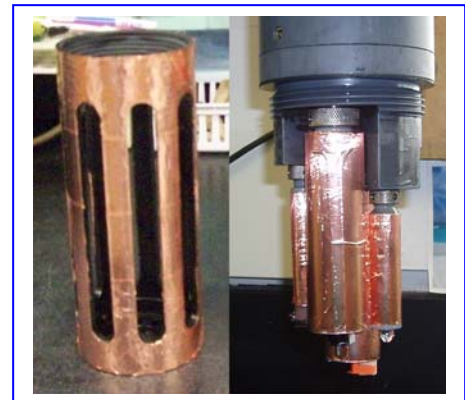
Figure 7.1 Copper tape on guard and probes
