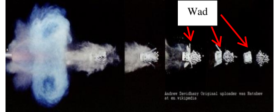
Figure 1. High speed photography of standard plastic wad.
