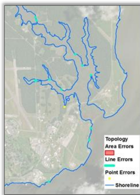
Figure 1. An example of an area with topological errors. The line errors indicate overlapping arcs and the yellow point errors show the location of disconnected arcs or dangles.
