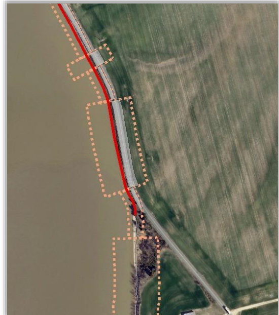
Figure 6. Shoreline shown in red has been coded for roads. The dashed lines indicate the bank height buffer widths. The shoreline should be coded for roads if the road intersects the bank buffer.
