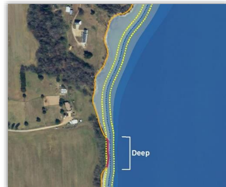
Figure 10. Bathymetry. The dashed yellow lines represent the 10m buffer around the - 1m bathymetric contour line. Where the buffer intersects the shoreline, the bathymetry is considered deep.
