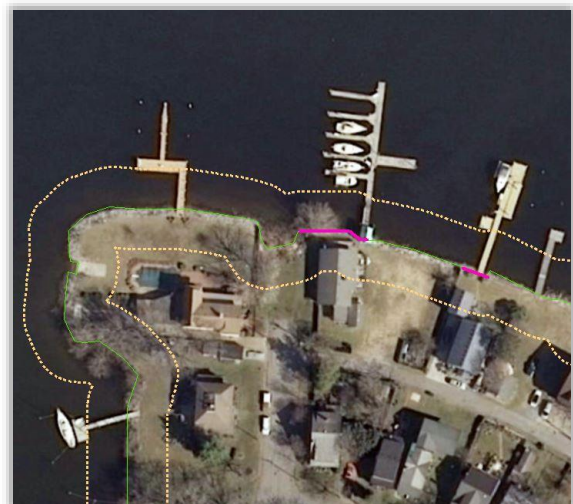
Figure 7. Permanent Structures (shown in bright pink) have been traced on the shoreline. The dashed lines indicate the bank height buffer widths. Trace the shoreline parallel to the permanent structure that is within the bank buffer.
