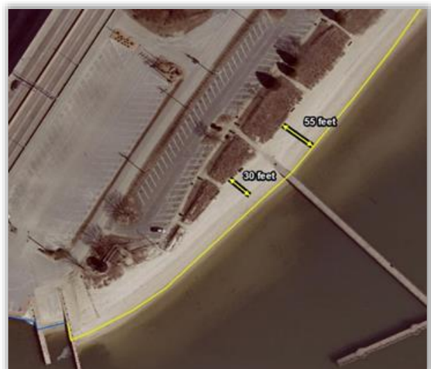
Figure 9. Wide beach showing a measured distance of 30 feet from dune grass to high tide line.
