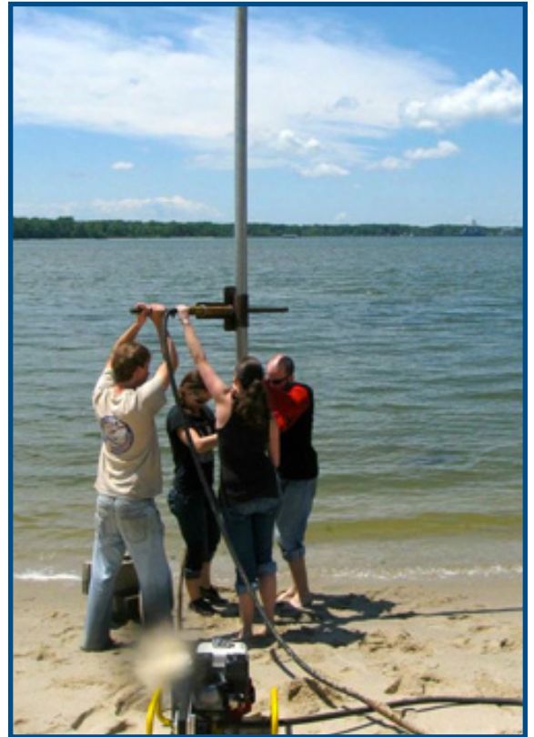
These researchers aren't tipping the goal posts after a big win. Instead, they are using a vibracorer to study groundwater entering the York River from beneath the VIMS beach. Photo by Mary Goodwyn
