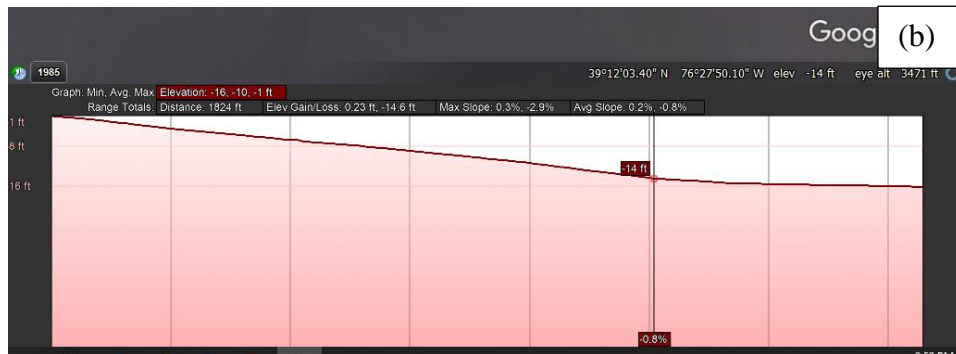
Figure 3: (a) The Google Earth view of the proposed outfall location and the cross-section bathymetry profile within 1000 feet (b) In 1200 feet, the depth increased from 10 to 14 feet
