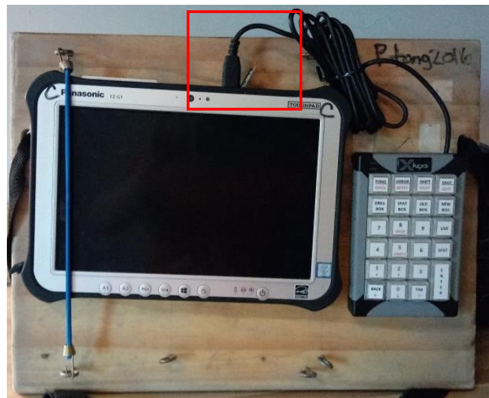
Figure 4: Tablet with keypad hooked up (USB cord from keypad plugged into the USB port on the top of the tablet). Notice the bungee connected to the eyehooks on the left side of the tablet.
