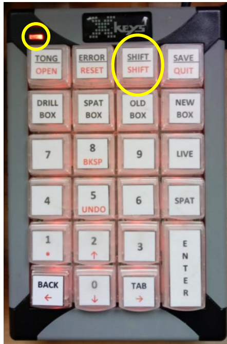
Figure 8: Secondary layer on the keypad. Notice that the backlight is red and the light in the upper left-hand corner is red. The function of each key in this layer is labeled in red. The shift key allows you to go back and forth between the two layers.
