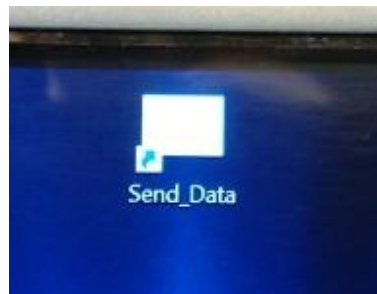
Figure 19: Send_Data icon located on the tablet’s desktop. Double tapping this with the stylus will prompt the tablet to send any new data files to the back-up computer.
