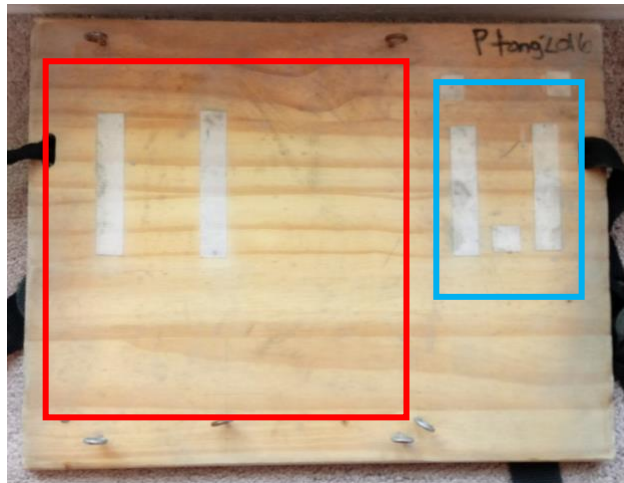
Figure 3: The wearable device without the tablet and keypad attached. The tablet connects to the Velcro in the red box, the keypad connects to the Velcro in the blue box. The keypad can be moved around to find the position that is most comfortable for the user.
